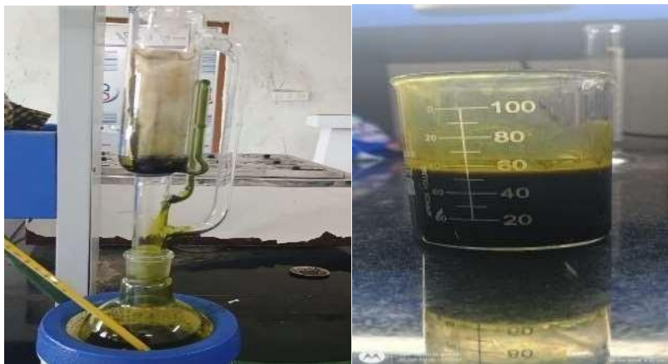
Figure 1: On going process of extraction in a Soxhlet apparatus.
